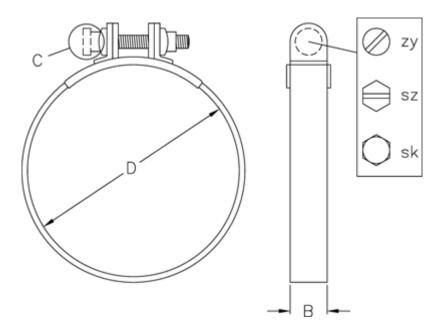
$C ext{ (screw type)} = SK$  Diameter D = 140Width B = 25
